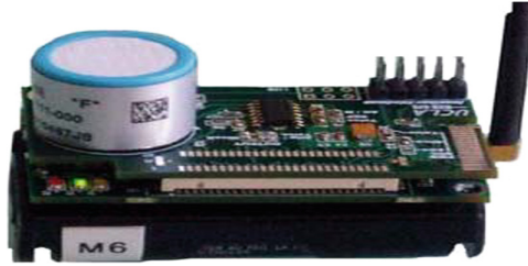
Fig. 4. The SewerSnort gas sensor board with a MicaZ mote [29]
